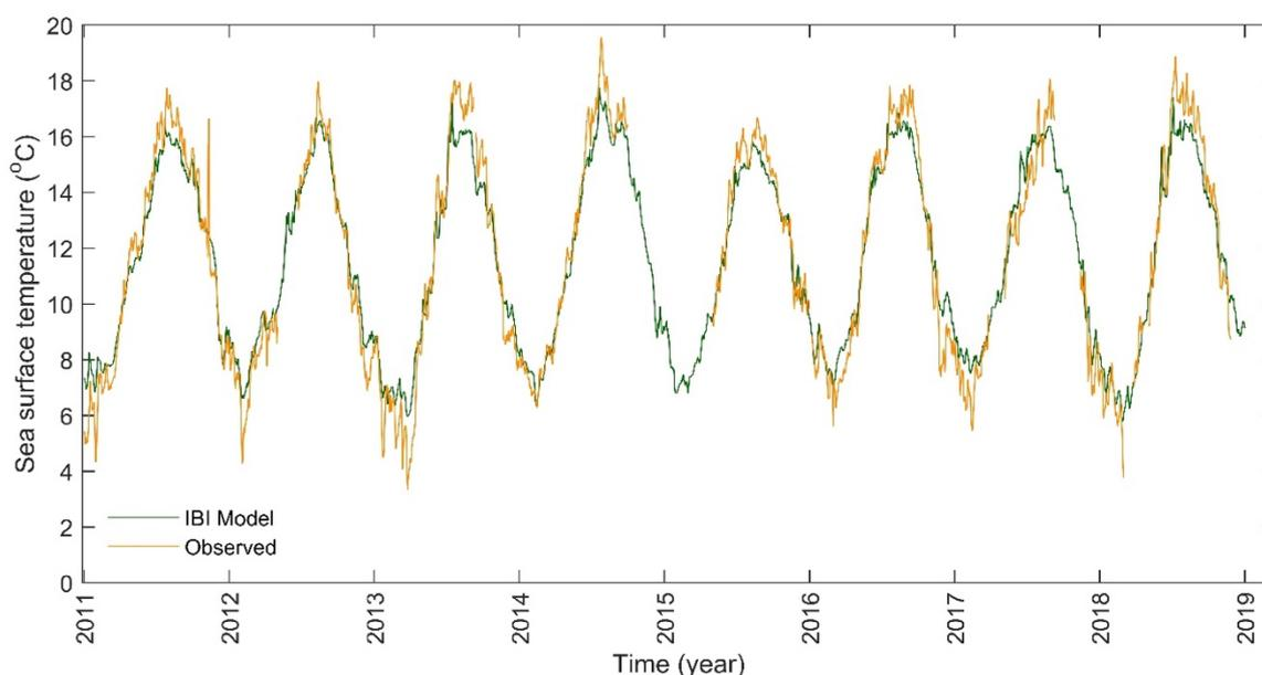
**Figure 8** Menai Strait sea surface temperature from January 2011 to January 2019. Temperature logger data from Menai Bridge Pier ('observed') is plotted in orange and IBI reanalysis/forecast temperatures ('modelled') are plotted in green.
